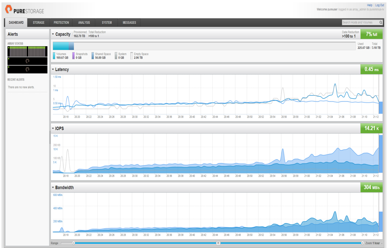
Figure 28: Pure Storage Dashboard during two UCS server cluster VSImax testing
